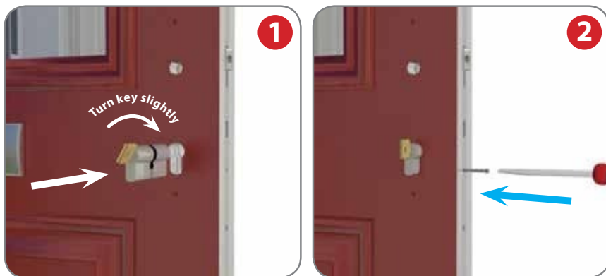
1. Insert cylinder and turn the key slightly. 2. Insert screw and tighten.
