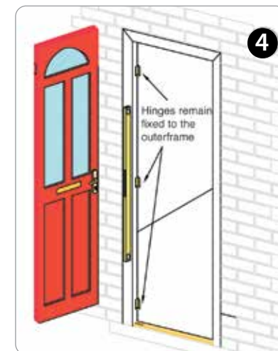
4. The leaf may be removed from the frame to ease installation. Final adjustments to frame position may be necessary when using fixed hinges. Once square and plumb, fix as per instructions. (See fixing positions)
