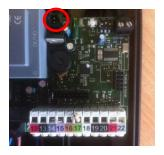
Screw the buzzer through one of the glands on the bottom of the control panel housing
