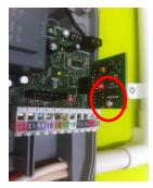
Now press the white button on the bottom slat transmitter for 2 seconds
