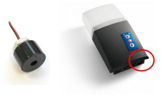
Press the white MEM/DEL button in your control panel 6 times and hold on the 6<sup>th</sup> press (top right – next to the dip switches) – you will hear a long beep.
